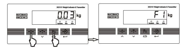
2. Press [PT] button, indicator shows "CAL X", "X" means the previous calibration method.
